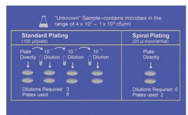
The Autoplate creates a 4-log dilution effect (20  $\mu$ l exponential mode) eliminating the need for four 10-fold dilutions.
